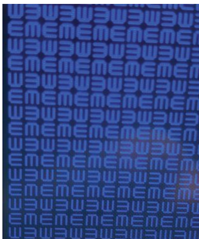
↑ 4K 18Gbps "ME" test pattern uncompressed on Quantum Data 980.
